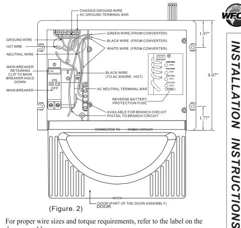
For proper wire sizes and torque requirements, refer to the label on the door assembly.
